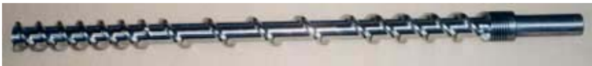
Fig. 11: Screw design of a flight progressive screw for silicone rubber extrusion
