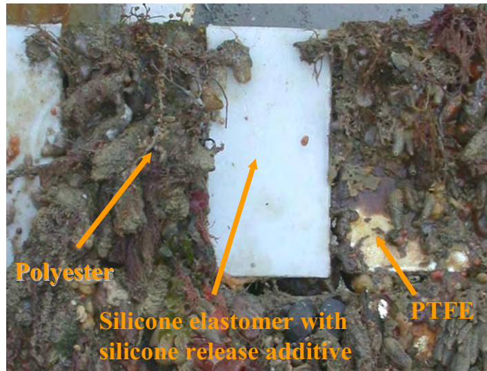
Figure 11. Extent of fouling of coated steel panels submerged for two-and-a-half years in the English Channel. Picture courtesy Dow Corning Ltd.
