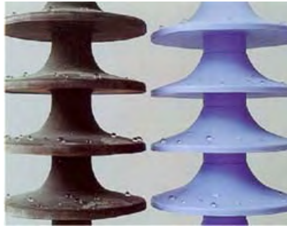
Figure 24. Comparison of an insulator after 23 years of use and exposure to pollution (left) vs. a retained sample kept at RT (right). Both still show excellent hydrophobicity as indicated by the high contact angle of the water droplets. (Picture courtesy of Lapp Insulators GmbH & Co.KG).
