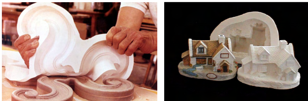
Figure 16. Flexible one-piece block molds: a silicone mold being separated from a PU copy (left); a silicone mold, and two copies, one after and one before finishing (right). Pictures courtesy of Dow Corning.
